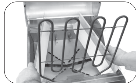
Fig. 22-3 Remove side liners
